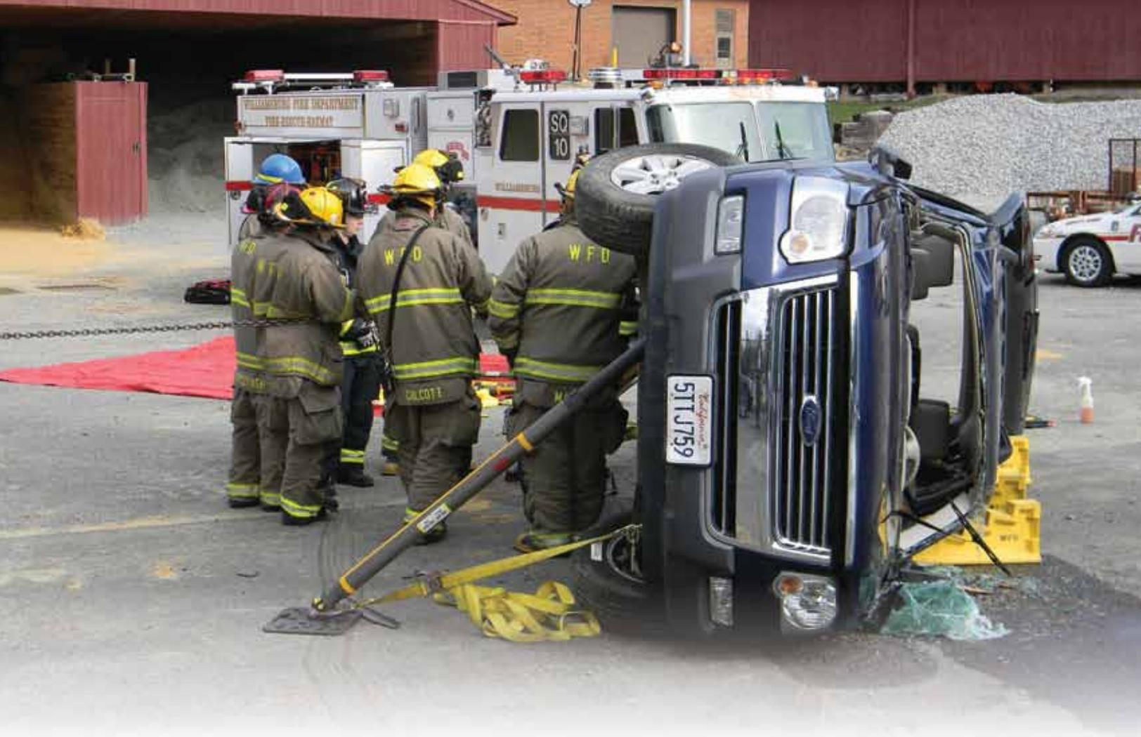
The City of Williamsburg Fire Department is now utilizing a vehicle stabilization kit in rescues where there is a potential for vehicle shift or rollover, to allow rescuers to focus on the extrication and treatment of passengers.
