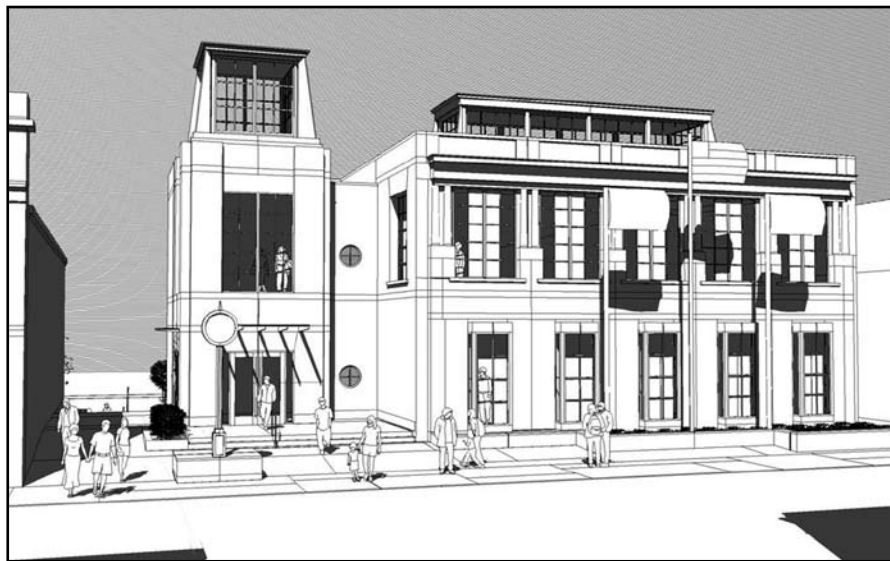
Although the building will be three stories, the façade on Main Street will be perceived as only two stories, designed to be in keeping with the scale of other commercial façades on Main Street.
